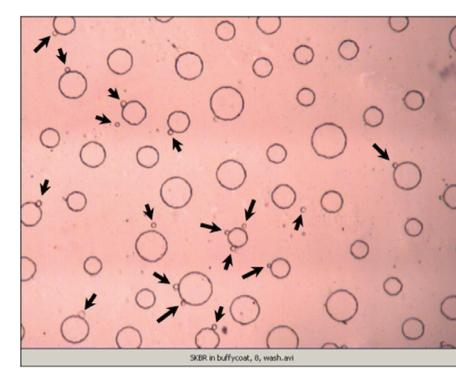
Visible light microscopic view of channel through coverslip showing the random array of posts and the SKBR3 cells which have been captured (arrows)
